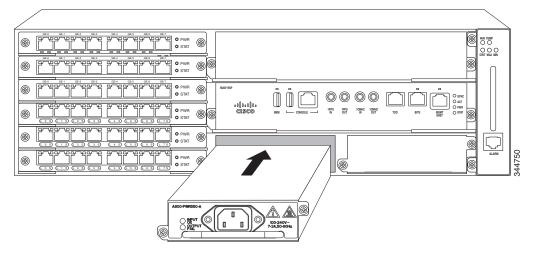
Step 4 Tighten the captive installation screws of the power supply. The recommended maximum torque is 5.5 in.-lb (.62 N-m).
